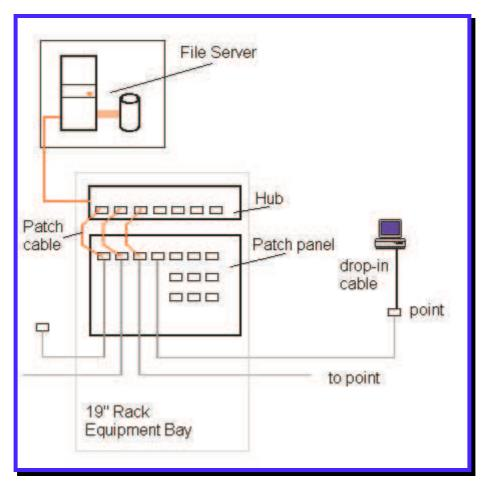
The connection between server and hub may be coax cable, twisted pair or even fibre optic cable. The short patch cables (< 0.5m) are used to connect the 'ports' of the hub to the patch panel connectors. The inside connection of the patch panel connector is wired to the rear of the bay and out to the respective point on the network. A short length of cable (< 10m) is used to connect the workstation to the point in the office.
