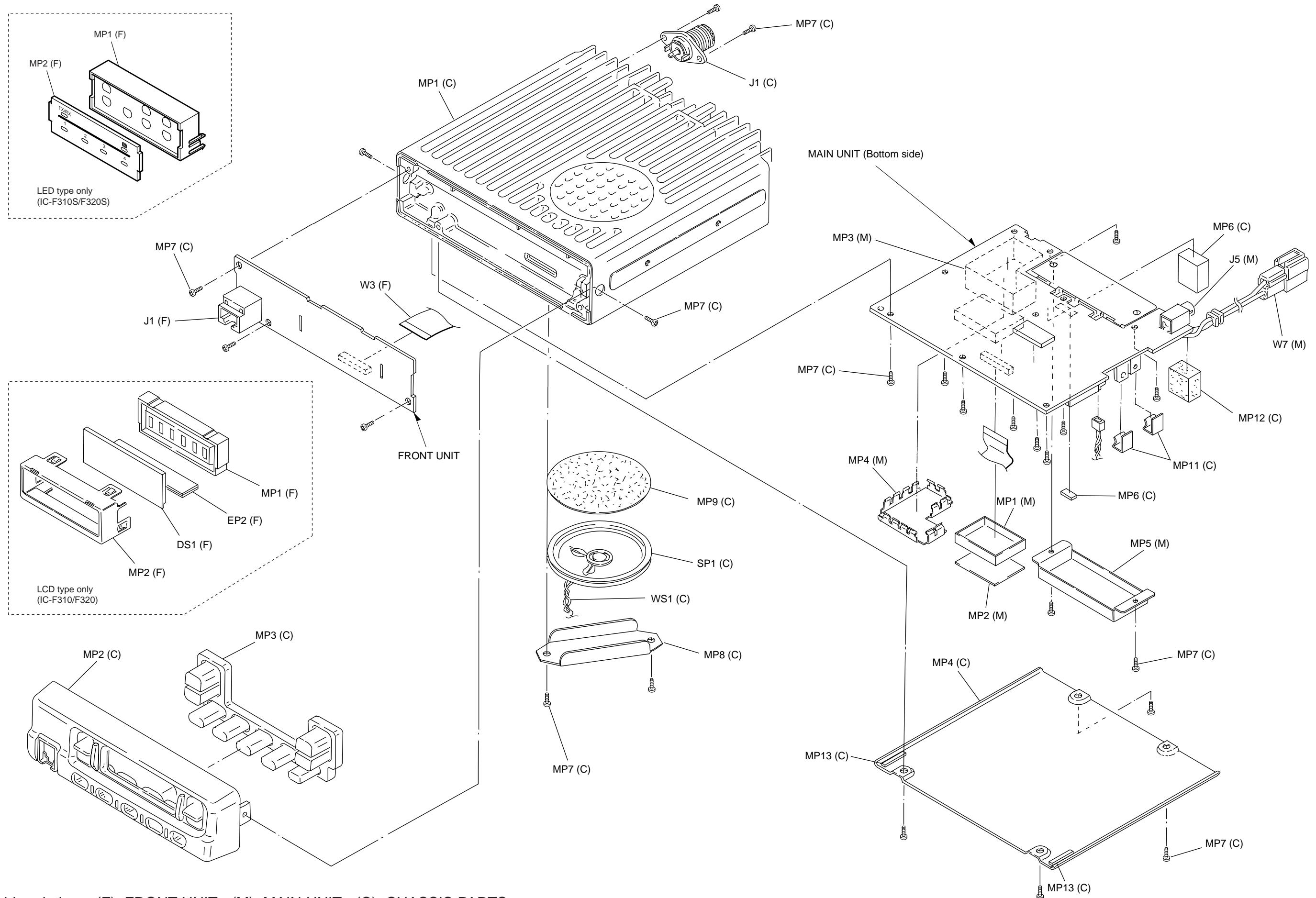
Unit abbreviations (F): FRONT UNIT (M): MAIN UNIT (C): CHASSIS PARTS
